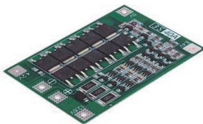
Фиг. 5. BMS (Battery management system)
